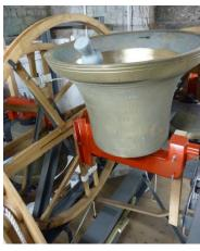
The bells are 'raised' so that the bell mouth faces upwards, and a simple mechanical design allows the bell to rest in this upside-down position.
