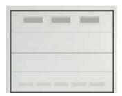
Overlap door, W 3270 x H 2580 with 3 rectangular ventilation grids in the upper panel and 5 rectangular ventilation grids in the lower one.
